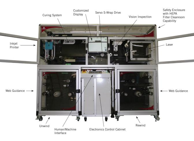
Small Footprint — In addition to its modular design, the Profection Series offers value as a turnkey solution with a much smaller footprint than systems utilizing subtractive processes. The in-line system is enclosed within a HEPA clean environment that allows for operator safety and cleanroom level processing without incurring added costs to prepare a facility level cleanroom.
