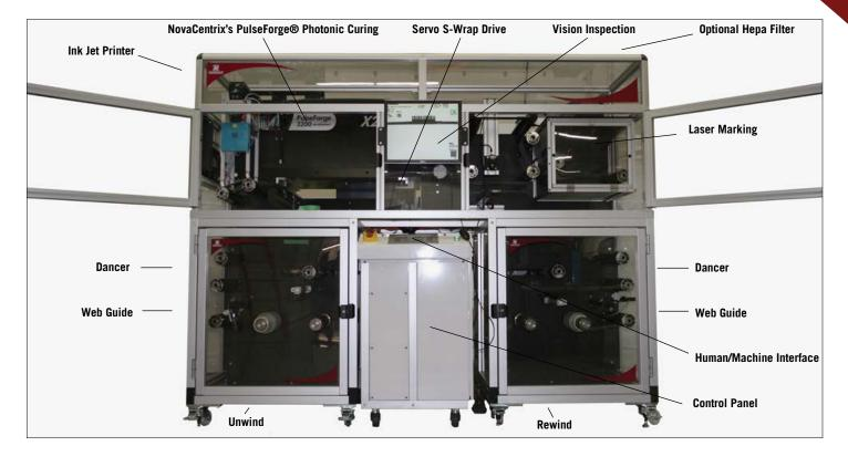
Small Footprint — In addition to its modular design, the Profection Series offers value as a turnkey solution with a much smaller footprint than systems utilizing subtractive processes. The in-line system is enclosed within a HEPA clean environment that allows for operator safety and cleanroom level processing without incurring added costs to prepare a facility level cleanroom.
